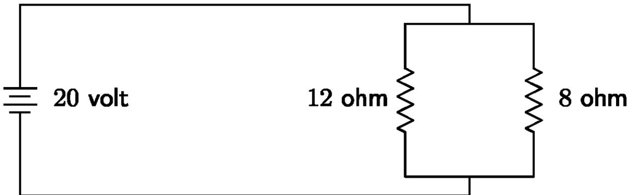
the electric current through the battery is  $25/6$  amperes. Thus, the parallel portion is **equivalent** to a single resistor of  $20/(25/6) = 4.8$  ohms.
