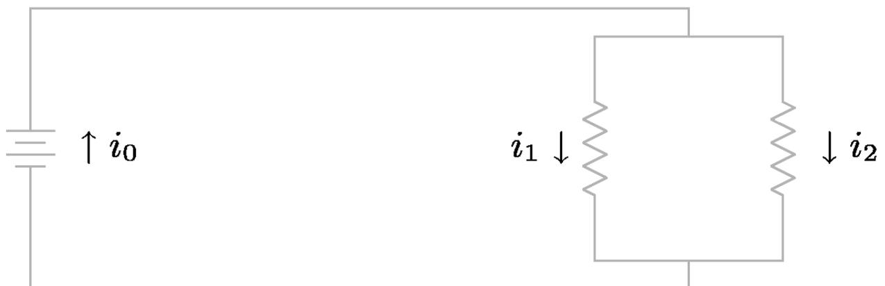
The Current Law, applied to the point in the upper right where the flow  $i_0$  meets  $i_1$  and  $i_2$ , gives that  $i_0 = i_1 + i_2$ . Applied to the lower right it gives  $i_1 + i_2 = i_0$ . In the circuit that loops out of the top of the
