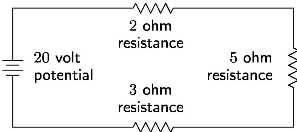
By Kirchhoff's Voltage Law, because the voltage rise is 20volts, the total voltage drop must also be 20volts. Since the resistance from start to finish is 10ohms (the resistance of the wires is negligible), we get that the current is  $(20/10) = 2$ amperes. Now, by Kirchhoff's Current Law, there are 2amperes through each resistor. (And therefore the voltage drops are: 4volts across the 2ohm resistor, 10volts across the 5ohm resistor, and 6volts across the 3ohm resistor.)
