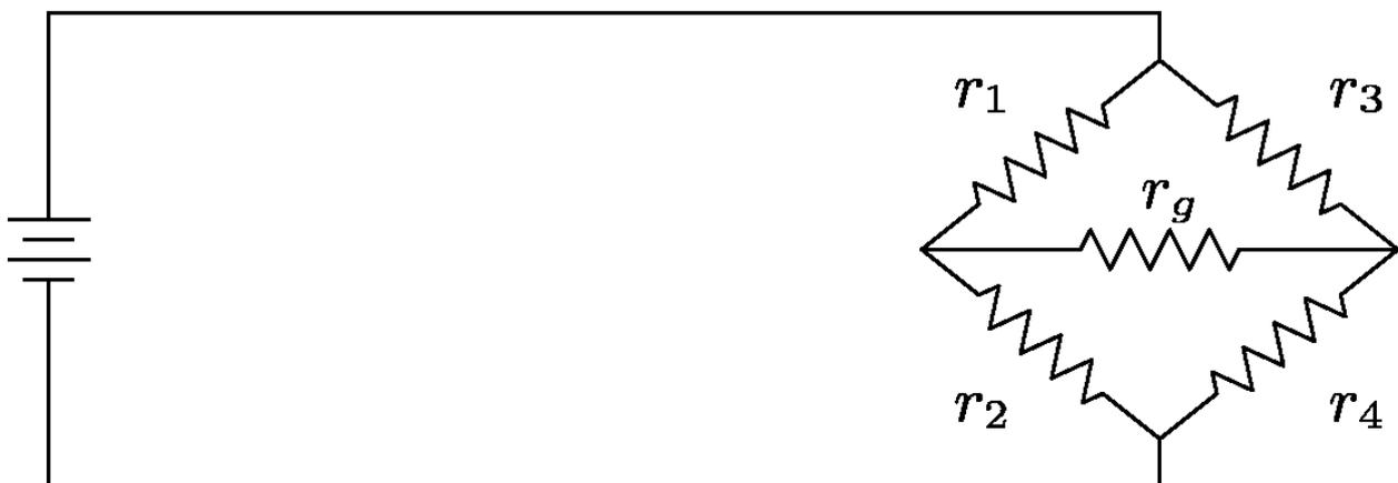
$r_2/r_1$  equals  $r_4/r_3$  if and only if the current flowing through  $r_g$  is zero. (The way that this device is used in practice is that an unknown resistance at  $r_4$  is compared to the other three  $r_1$ ,  $r_2$ , and  $r_3$ . At  $r_g$  is placed a meter that shows the current. The three resistances  $r_1$ ,  $r_2$ , and  $r_3$  are varied— typically they each have a calibrated knob— until the current in the middle reads 0, and then the above equation gives the value of  $r_4$ .)
