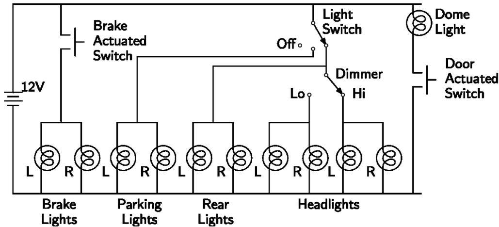
The designer of such a network needs to answer questions like: How much electricity flows when both the hi-beam headlights and the brake lights are on? Below, we will use linear systems to analyze simpler versions of electrical networks.
